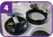
Remove the filter lock ring and lid.
