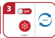
Turn pump 1 off by pressing the pump one icon once. Repeat steps 2 and 3 until air is removed from pump 1 and water is coming from jets.
