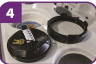
Remove the filter lock ring and lid.
