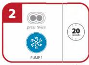
Turn pump 1 on high speed for 20 seconds by pressing the pump icon twice.
