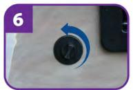
Loosen (do not remove) the air bleeder valve by turning counterclockwise.
