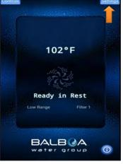
Selecting "Controls" will open a list of installed components like pump(s), blower, lights, etc.
