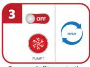
Turn pump 1 off by pressing the pump one icon once. Repeat steps 2 and 3 until air is removed from pump 1 and water is coming from jets.
