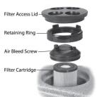
**NOTE:** Make sure the o-ring is on the air relief valve, and is finger tight prior to starting the pump. This o-ring should periodically be lubricated with a silicone lubricant.
